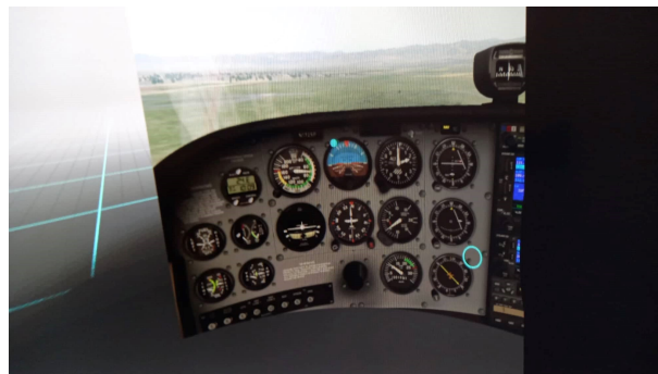
Figure 3. Experienced pilot gaze point (the solid circle) and a young pilot gaze point (the hollow circle) mapping from VR headset
